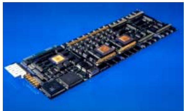
Fig. 5: Days of the past? A frame-grabber for machine vision with special-purpose processors. (Photo: Jan D. Martens)
