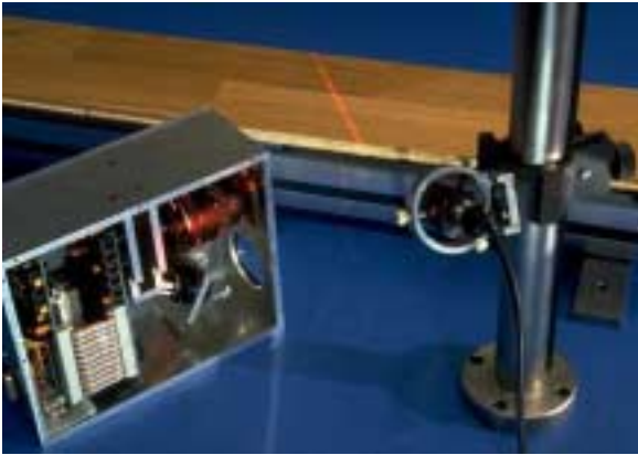
Fig. 4: Parquet-floorboard inspection by smart camera (Photo: Jan D. Martens)
