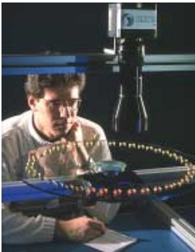
Fig.3: Inspection of air-brake fittings at Raufoss AS using a telecentric lens. (Photo: Jan D. Martens)
