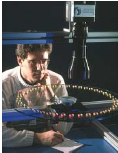
Figure 6: Inspection of air-brake fittings at Raufoss AS (Photo: Jan D. Martens)
