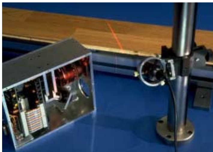
Figure 3: Parquet-floorboard inspection by smart camera (Photo: Jan D. Martens)
